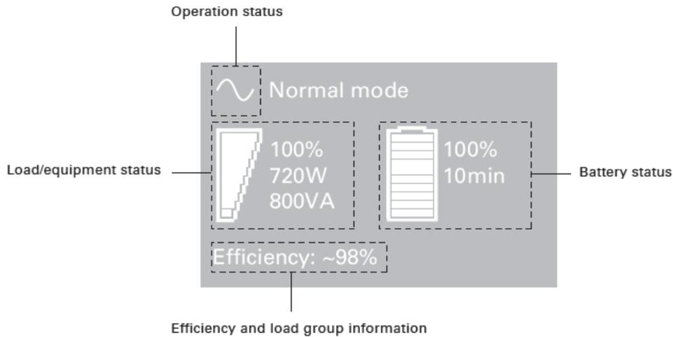
As default, or after 5 minutes of inactivity, the LCD displays the screen saver. The backlight LCD automatically dims after 10 minutes of inactivity. Press any button to restore the screen.
