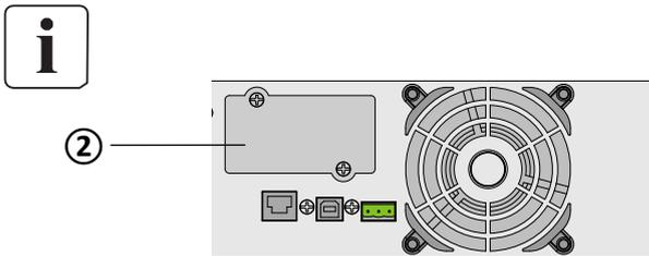
It is not necessary to shut down the UPS before installing a communication card
