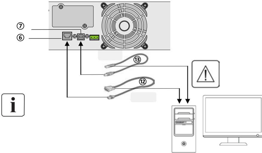
1. Connect the RS232 (12) or USB (13) communication cable to the serial or USB port on the computer equipment.
