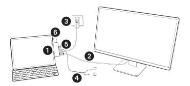
Connect the USB 3.2 Gen 1 Type-C male connector to your USB-C enabled device.
