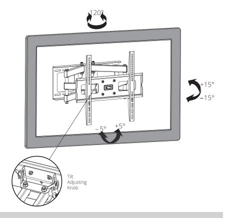
To adjust the tilt angle, loosen the Tilt Adjusting Knobs located behind the wall mount arm assembly plate. Once the display is at the desired position, retighten the knobs to hold.
