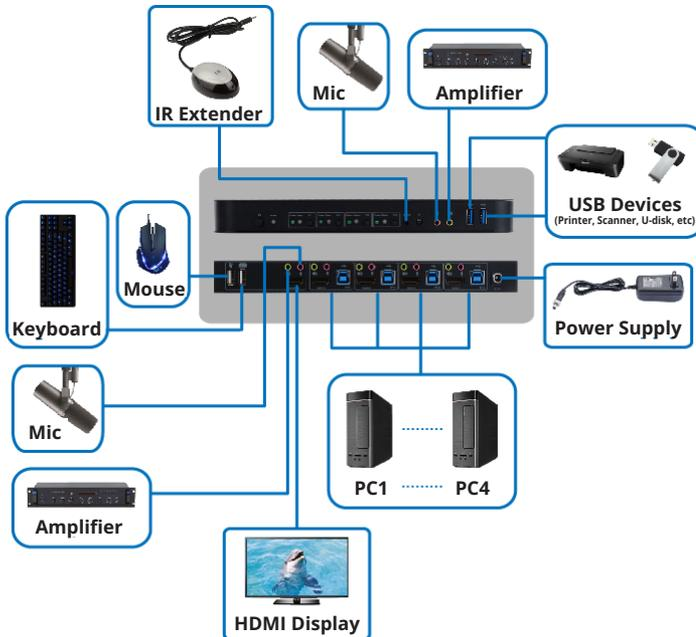
1. Connect computers to the USB-B input ports using USB cables. Connect the computers' microphone and stereo audio ports using 3.5 mm audio cables. Connect computers to the "HDMI In" ports using HDMI cables.
