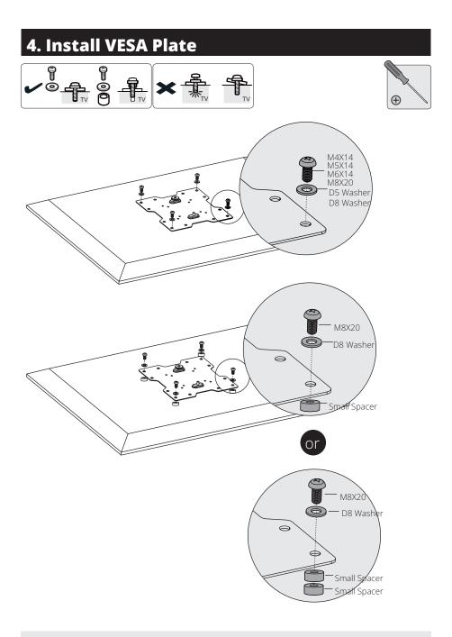
**Note:** Firmly secure the VESA plate to the display using the appropriate screws, washers and spacers (if necessary).
