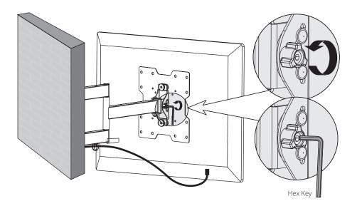
You may need to slightly loosen or tighten the adjustment screw using the supplied Hex Key depending on the weight of display installed.
