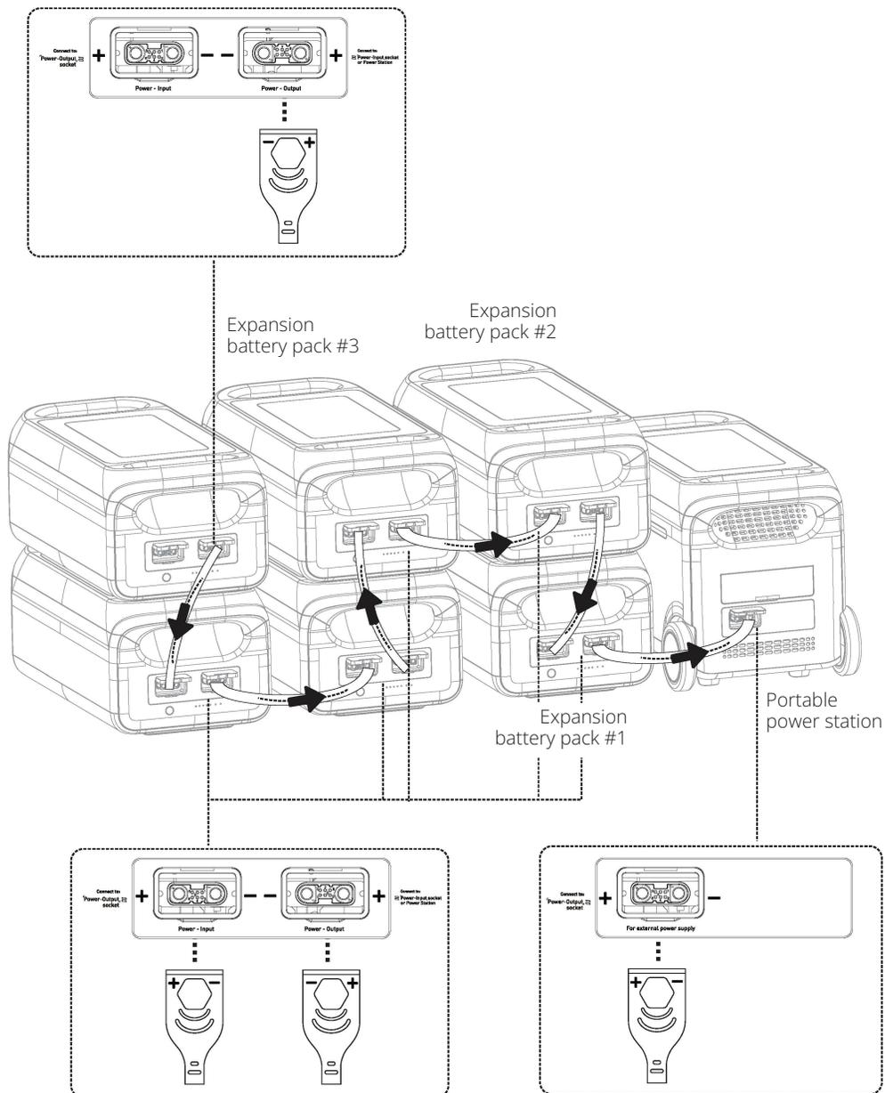
**Note:** + and - symbols are labeled on battery packs and cables to reduce reverse polarity connections.
