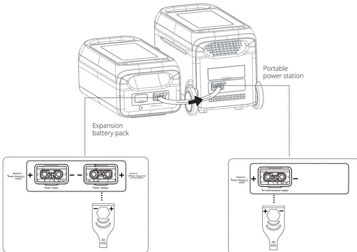
**Note:** + and - symbols are labeled on battery packs and cables to reduce reverse polarity connections.
