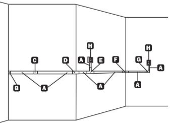
A Raceway Wiring Duct (N080-D25-2M-WH): 2-piece raceway wiring duct.
