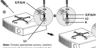
**Note:** Choose appropriate screws, washers and spacers (if necessary) according to the type of projector. Installers are responsible to provide hardware for other types of mounting situations.
