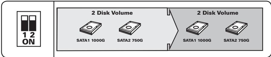
**JBOD Mode** – This mode combines the two hard drives into one large drive for the purpose of increased storage space. Data is stored on one drive at a time, so when the first one is full, the next one begins to be used. The computer's operating system will recognize them as a single drive.
