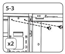
The rail attachment points are numbered to help you align each pair of rails at the same depth. Before attaching the rails using the screws (shown in Step 5-3), make sure the same number appears in all three windows. **Note: Number shown in Step 5-2 is for illustration purposes only; attach rails at desired depth.**
