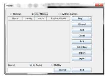
The User Macros page allows you to add macros to the unit that can be performed on the connected computer using the Macro List feature of the control panel (See Macro List section for details). By default, the User Macros page is displayed when the Hotkeys / Macros icon is clicked on. To display the page when it isn't selected, click on the User Macros button at the top of the Hotkeys / Macros screen.
