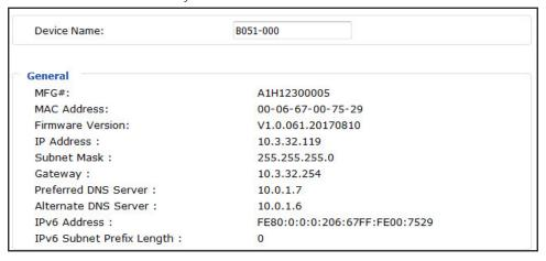
7. Click on the Network tab at the top of the screen. From here, a fixed IP address can be assigned in the same way as when using a web browser. (See steps 4 through 8 in the Web Browser section)
