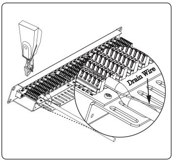
**3** Make sure the drain wire has good contact with the rear panel.
