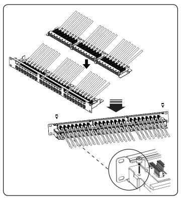
**7** Use the included screws to attach the cap and grounding wire.
