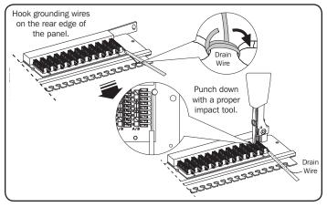
5 Make sure the drain wire is tied between the panel and the rear cable manager.
