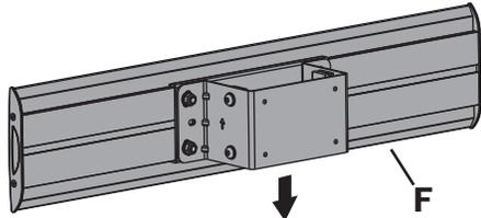
Slide the first universal plate onto the column, making sure the arrow on the universal plate is pointing up.
