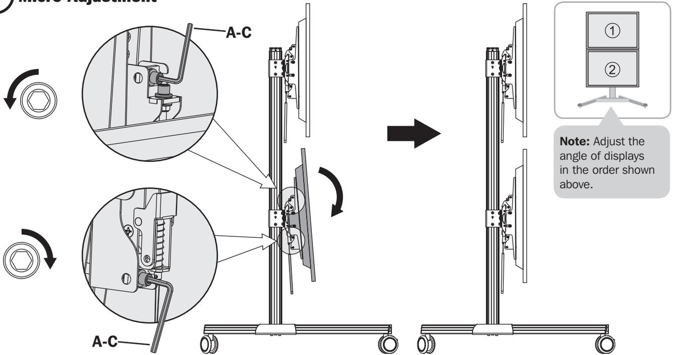
If the display tilts upward, adjust using the 5 mm hex key (A-C), as shown above.
