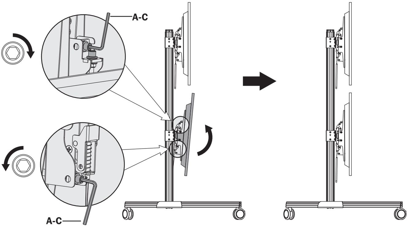
If the display tilts downward, adjust using the 5 mm hex key (A-C), as shown above.
