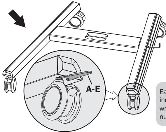
Each caster can be adjusted independently for fine tuning. Using the wrench (A-E), slightly turn each caster nut to lower or raise the base.
