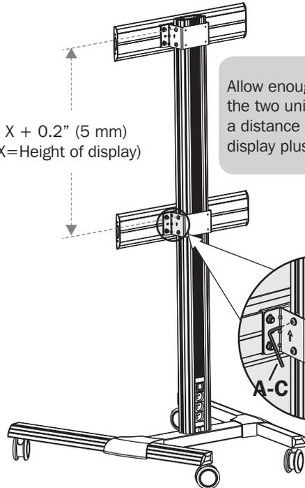
Once the universal plate positions have been determined, use the 5 mm hex key (A-C) to secure them to the column.
