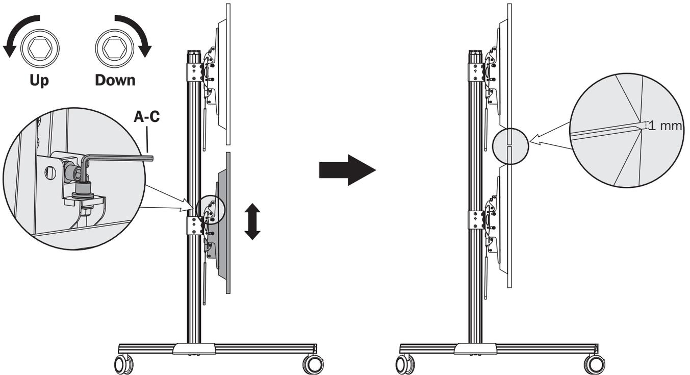
To move the displays up or down, adjust using the 5 mm hex key (A-C), as shown above.
