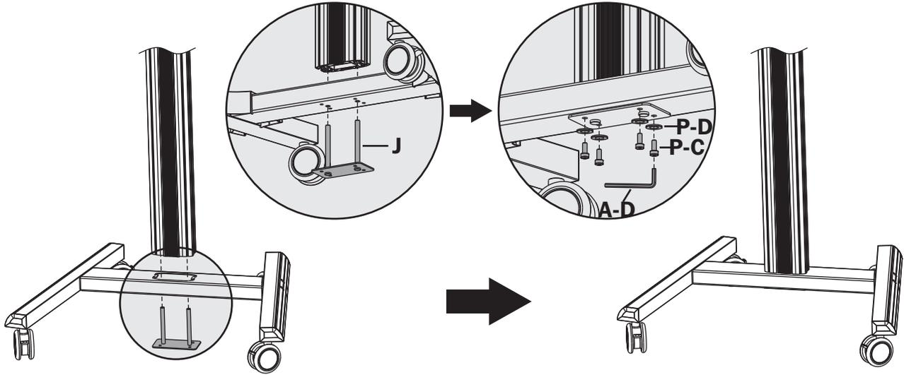
Insert the connecting piece (J) into the column to attach the column to the base. Use M8x35 screws (P-C), D8 washers (P-D) and the 6 mm hex key (A-D) to secure the connecting piece and column to the base.
