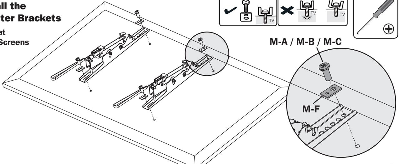
**Note:** Choose appropriate screws and spacers according to the type of screens.
