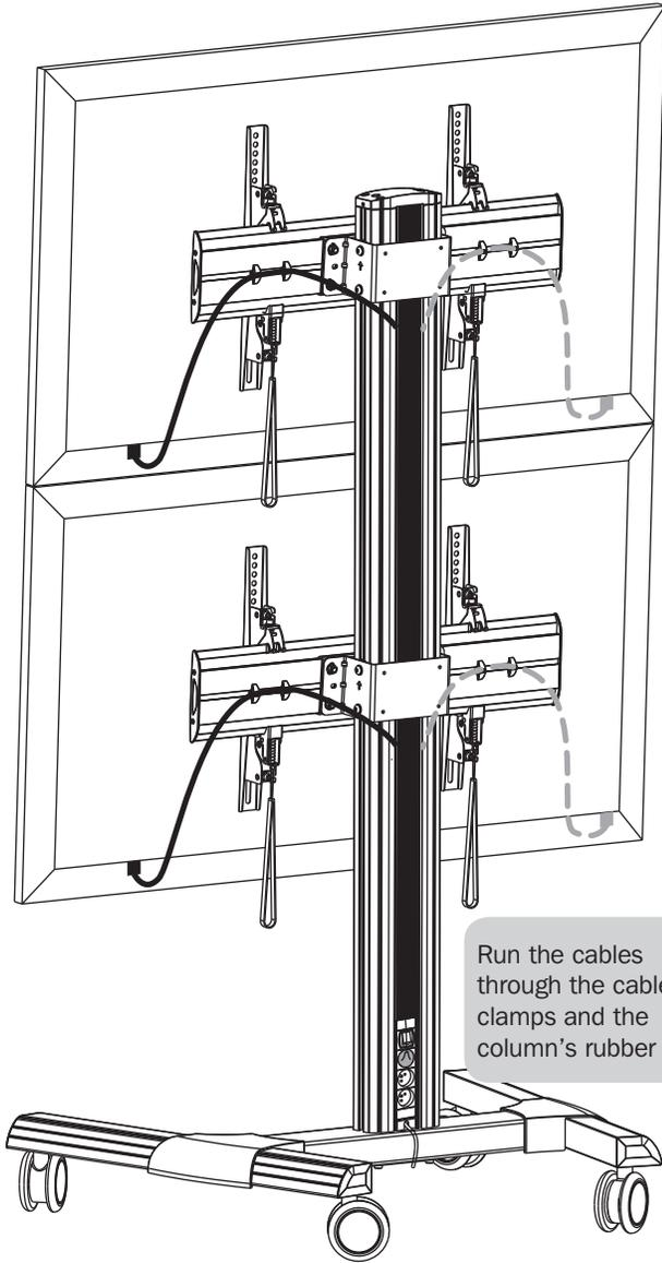
Run the cables through the cable clamps and the column's rubber strip.
