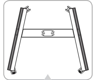
**Note:** Position base assembly with wheels facing forward.
