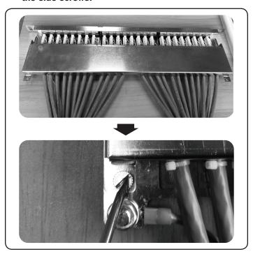
5 Attach the panel's grounding lug to a rack or cabinet.
