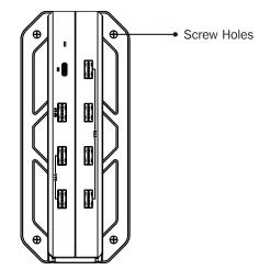
The U280-008-CQC-ST can be wall-mounted using the included screws and the stand.
