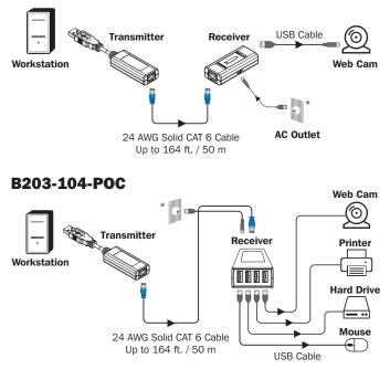
\* When connecting the receiver to high-power device(s), add external power via its USB Micro-B port.
