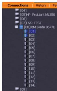
For HP blade servers, associations are made on a blade by blade basis. Each blade is associated with a single port. To access a blade, click on its port entry in the tree.
