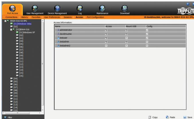
When the master KVM switch is highlighted in the port list, the *Access* sub-section displays only one setting column; Config. When a port is highlighted in the port list, the *Access* sub-section displays three settings columns; Access, Mount USB and Config. The section that follows describes these settings, and how to edit them.
