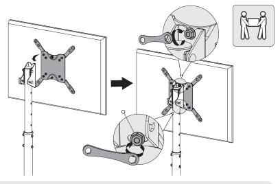
Use the included wrench to secure the VESA plate and display to the vertical support. Make sure the display is secure before releasing.
