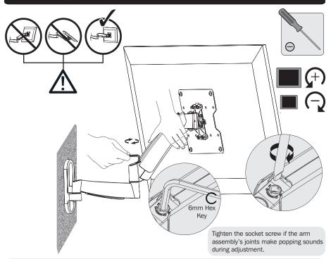
Keep the wall mount arm level during tension adjustment. You may need to slightly loosen or tighten the adjustment screw using the provided Hex Keys depending on the weight of display installed.
