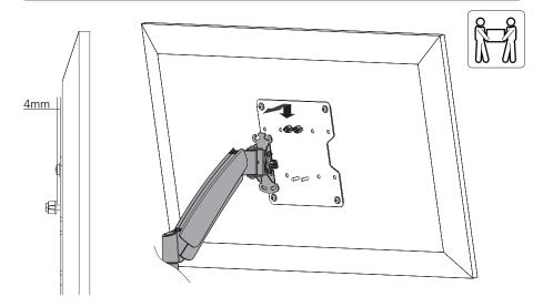
Using an assistant or mechanical lifting equipment, lift the display with attached VESA plate. Set the VESA plate's upper thumbscrews over the top flange of wall plate arm. Make sure the VESA plate's lower screws fit inside of the wall plate arm's lower hole.
