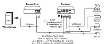
For the B203-101/104-IND models only: when connecting power-hungry device(s), use either the included external power supply or RS-232 Phoenix connector to add external power.
