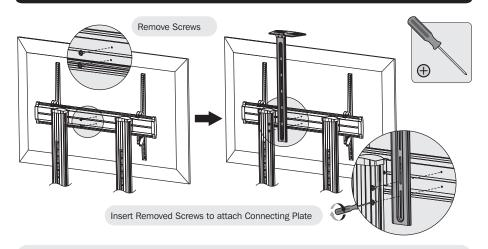
Remove the Universal Plate's two rear screws, then attach the Camera Shelf Assembly using the same screws just removed. Adjust the Camera Shelf Assembly to the desired height, then secure by tightening the screws with a Philips screwdriver.
