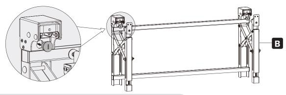
Remove caps before installing the pop-out module.
