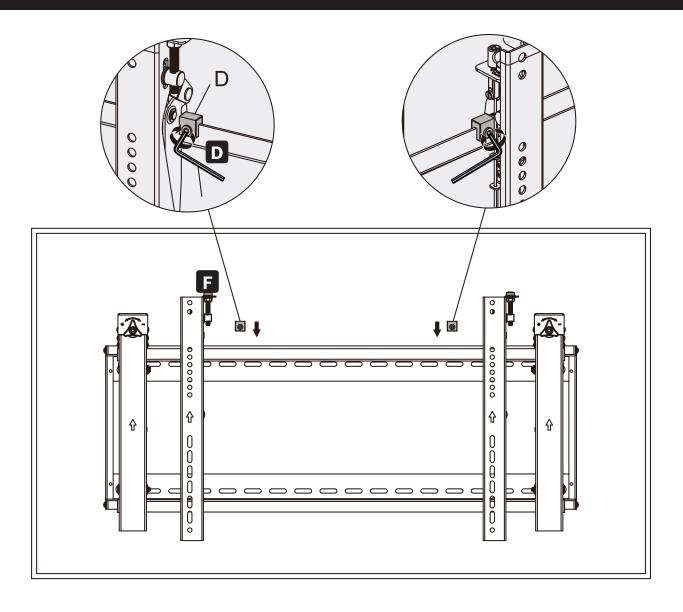
Install both of the anti-skid blocks as close to the adapter brackets as possible.
