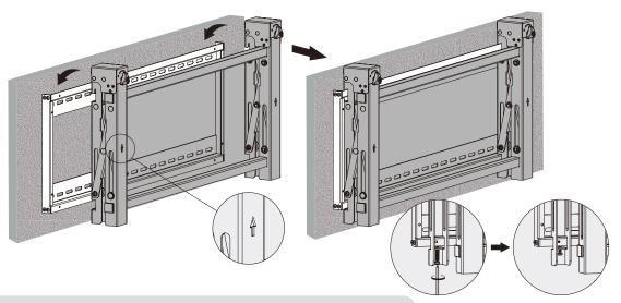
Hang the pop-up module onto the wall plate. Secure it by tightening both screws.
