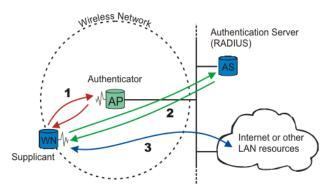
When the client provides the login credentials, the Switch sends an authentication request to a RADIUS server. The RADIUS server validates whether this client is allowed access to the port.
