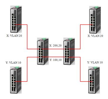
This example shows how to configure switch A with ports 1 on the Switch to tag incoming frames with the service provider's VID of 200 (ports are connected to customer X network) and configure port 7 to service provider's VID of 100 (ports are connected to customer Y network). This example also shows how to set the priority for port 1 to 3 and port 7 to 4.
