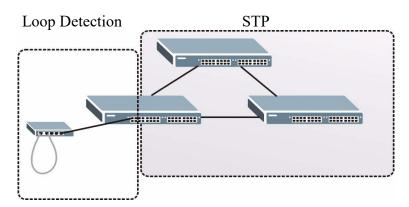
The loop detection function sends probe packets periodically to detect if the port connect to a network in loop state. The Switch shuts down a port if the Switch detects that probe packets loop back to the same port of the Switch.
