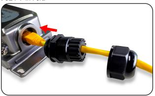
**Step 2:** Turn clockwise to tighten the **gland body** with the Outdoor PoE Extender.
