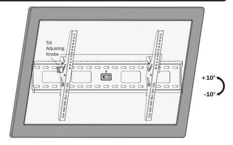
To adjust the tilt angle, loosen the Tilt Adjusting Knobs located on the sides of the adapter brackets. Once the display is at the desired angle, retighten the knobs to hold.
