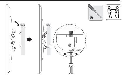
Using an assistant or mechanical lifting equipment, hook the display with attached adapter brackets over the top of the mounted wall-plate. Tighten the two bolts on the bottom of the adapter brackets to secure the unit.
