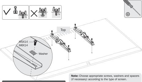
2-2 For Recessed Back Screen, Curved Screens or to Access A/V Inputs
