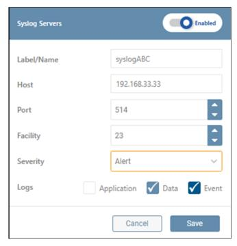
Figure 4-62: Adding and Deleting a Syslog Server
