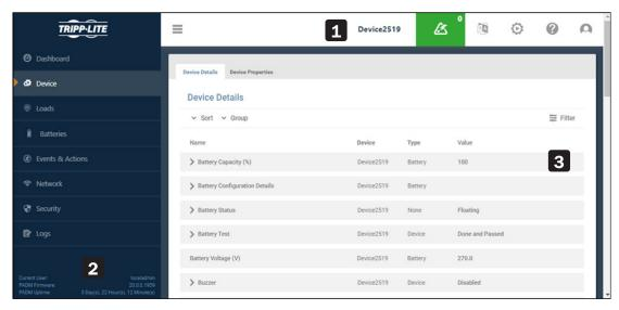
Figure 3-3: PADM Web Interface Main Sections
