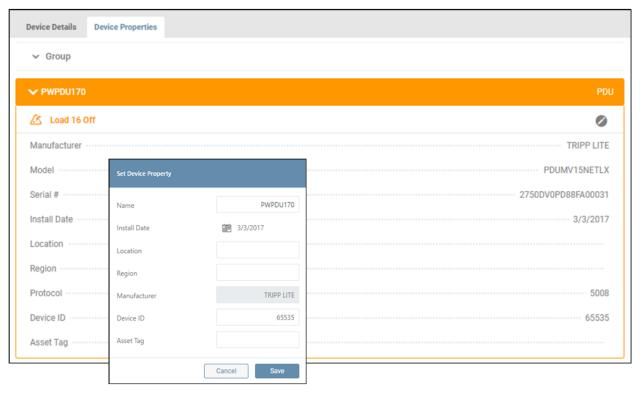
Figure 4-8: Displaying and Editing Device Properties
