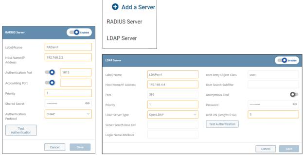
Figure 4-43: Adding a RADIUS Server and an LDAP Server
