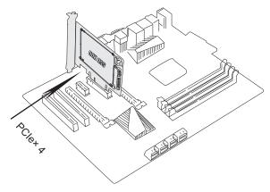
7. Fix the full profile bracket to the tower rear panel of the PC and screw tightly to secure connection.
