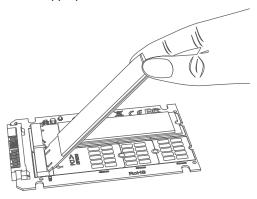
2. Secure the SSD into place using the included SSD mounting hardware.
