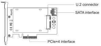
Secure the P970-U2M2 into place with the PCE-U2-PX4 using the mounting hardware that is included with the PCE-U2-PX4 (sold separately)
