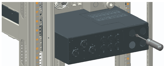
Figure 4. Remove the Wire Access-Point Covers
