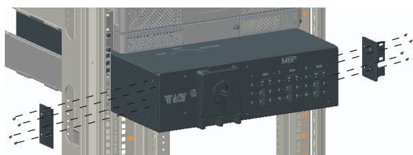
Figure 6. Install the Mounting Ears
