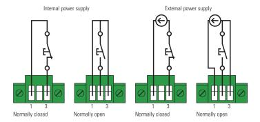
Terminal wire size rating is 0.32-4 mm2 (22-12 AWG). Suggested wire size is 0.82 mm2 (18 AWG).
