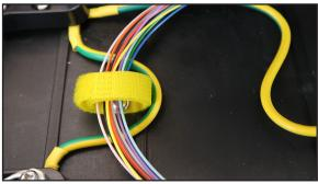
Figure 1-15: Manage cable with magic band tie
