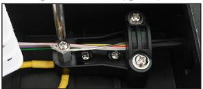
Figure 1-26: Attach the strength member
