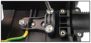
Figure 1-23: Remove the press clamping
