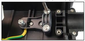
Figure 1-7: Remove the upper clamping
