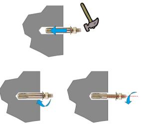
Figure 2-7: Install the expansion bolt
