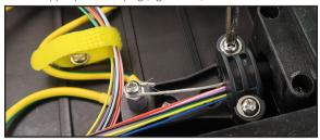
Figure 1-12: Secure the upper press clamping
