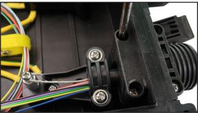
Figure 1-13: Secure the wedge
