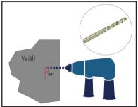
Figure 2-5: Drill holes in the wall
