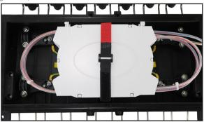
Figure 1-33: Close the splicing tray cover
