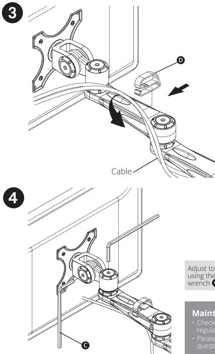
Adjust torque if needed using the included hex wrench **G**.
