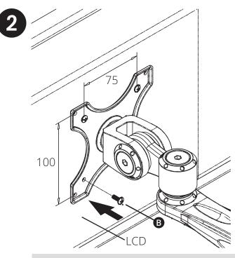
**Note:** Choose the appropriate screws, washers and spacers (if needed) according to the type of screen.
